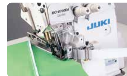
Rolling in tape MO-6745DA-FF4-360/N077 (N077: Clean finish top and bottom)
