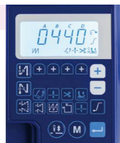
Operation panel for the sewing machine without thread trimmer
