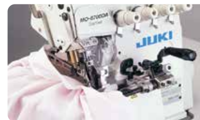
Gathering MO-6714DA-BE6-327/S162 (S162: Swing-type gathering device, manual-lever operated)
